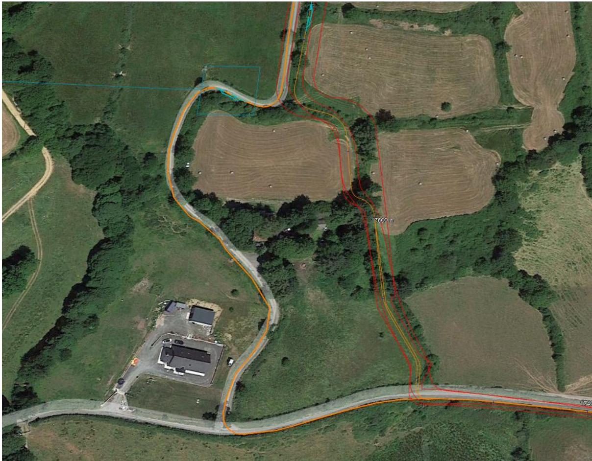
Figure 4-4 Section of the proposed grid connection (on right) and original layout on left
